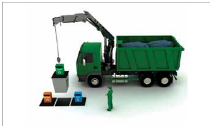
RAISING UNDERGROUND WASTE BIN
