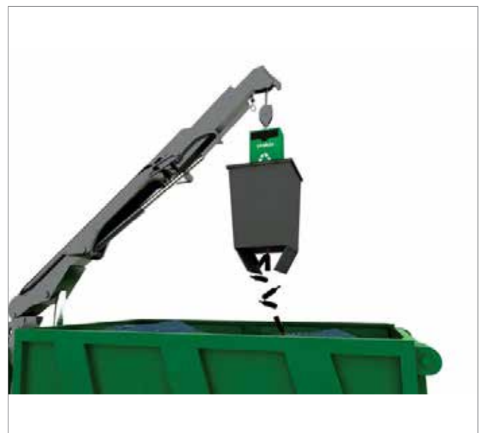
WASTE BIN DISCHARGE METHOD
